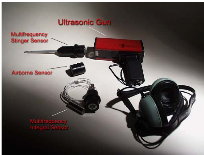
Figure 4. Ultrasonic system with multi-frequency sensor.
