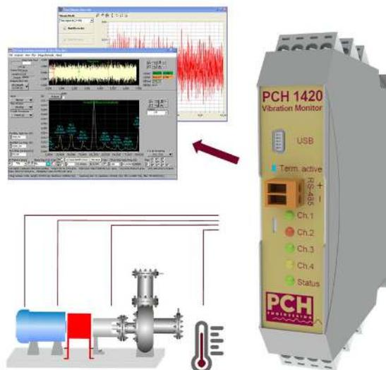
In the standard IEPE version, each vibration channel operates within 2 simultaneously running frequency bands. The bands are configurable from 0.7 Hz up to 11.5 kHz and will typically monitor the 10-1000 Hz area (ISO 10816-3), as well as the high frequency area 2-10 kHz, where roller bearing resonances are detected.
