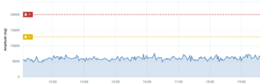
BL2 Dryer Fan Zone 1 right hand side - 3_Fan Shaft DE bearing (Sensor #3) - Peak-to-Peak
